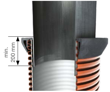
Correct installation of the telescopic pipe in the riser pipe of the chamber.
