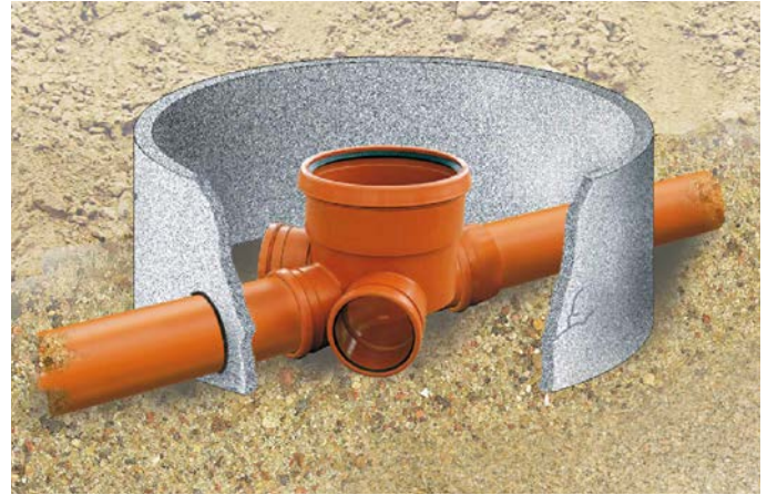
Example of use of a plastic chamber base during renovation of concrete chambers using the relining method
